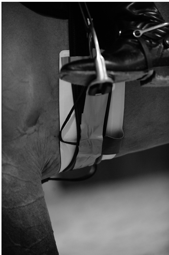
Fig. 1. The pressure mat positioned under a horse's girth during the study.
